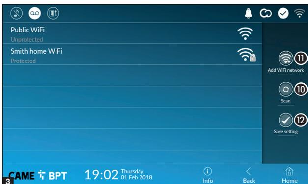
3 The page shows any detected networks; to manually scan for networks, touch this button 10.
