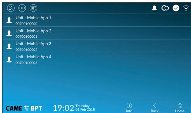
The window lets you view the credentials of the four users enabled to connect to the device via mobile devices.
