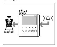
If an alarm contact connected to the relevant receiver entrance is activated, a signal is sent to the porter and an intermittent acoustic signal sounds on the receiver.
