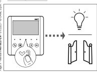
Press the AUX button to activate the desired auxiliary command, for example switching on a light or opening the gate.
