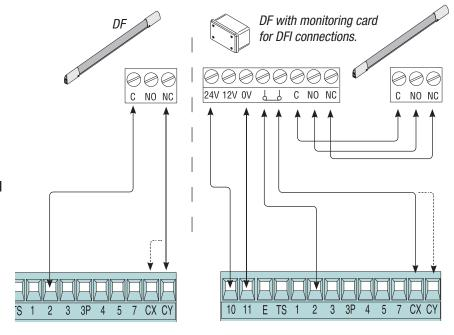
Electrical connection for running the photocells safety test
