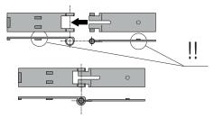
4) Insert the hinges into the box (either on the right or left side, as you prefer) and secure them using the supplied nuts and bolts.
