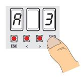
2) Select 1 and press ENTER to confirm, the automatic gate run calibration procedure...
