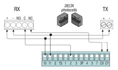
Configure either (N.C.) contacts CX or CY, input for safety devices such as sensate edges, that comply with
