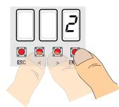
3) ...an available number between 1 and 25 will flash for a few seconds. This number will be assigned to the user after sending the code via transmitter or other command device.
