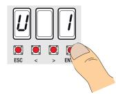
2) select command (1=step-by-step, 2=sequential, 3=open, 4=pedestrian / partial opening, 5= B1-B2 output contact) to assign to user via the greater-than and lesser-than arrows on the keyboard...
