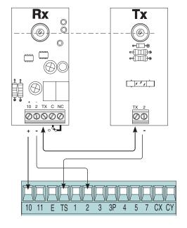
At each opening and closing command, the control board assesses the efficiency status of the safety devices (photocells). Any anomaly found is signaled with the flashing of the LED on the control board. Consequently it cancels any commands coming from the transmitter or the button.
