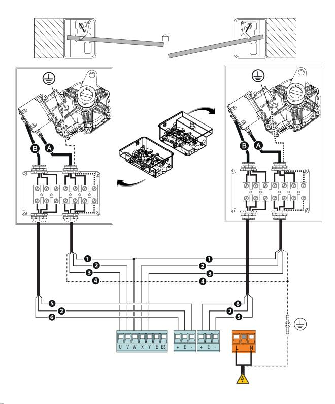
Check the correct direction of rotation of the gearmotor and, if necessary, invert the connection of the brown and black cables.
