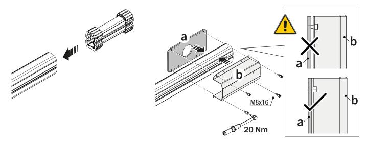
Fix the boom to the anchoring plate.
