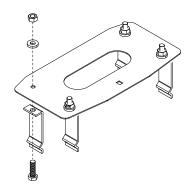
Fit the anchoring plate in the iron cage.
