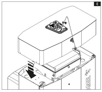
⚠ Connect the earth wire to the Faston terminal to be welded on the cover before closing it. See paragraph [Final operations].
