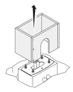
Fill the hole with soil around the concrete block.
