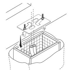
Position the anchoring plate, taking note of the measurements shown in the drawing.
