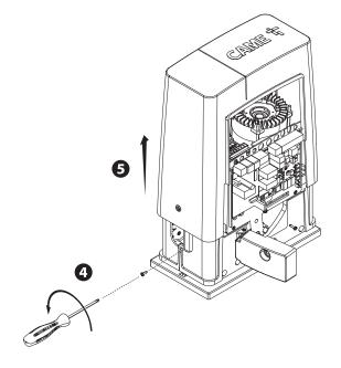
Place the operator on top of the anchoring plate.
