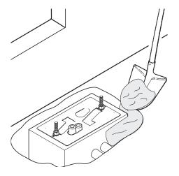
Insert the electrical cables into the tubes until they protrude by about  $600\ mm$ .
