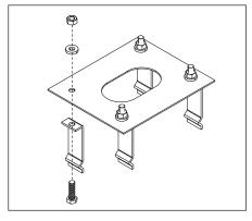
Fit the anchoring plate in the iron cage.
