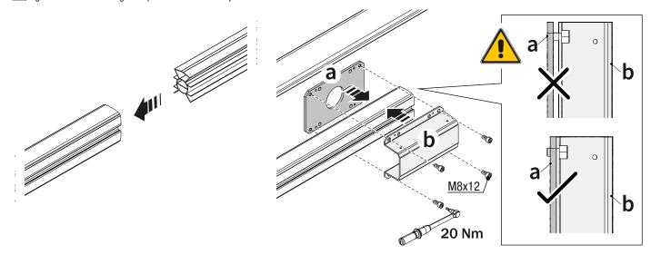
Fix the boom to the anchoring plate.
