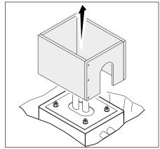
Fill the hole with soil around the concrete block.
