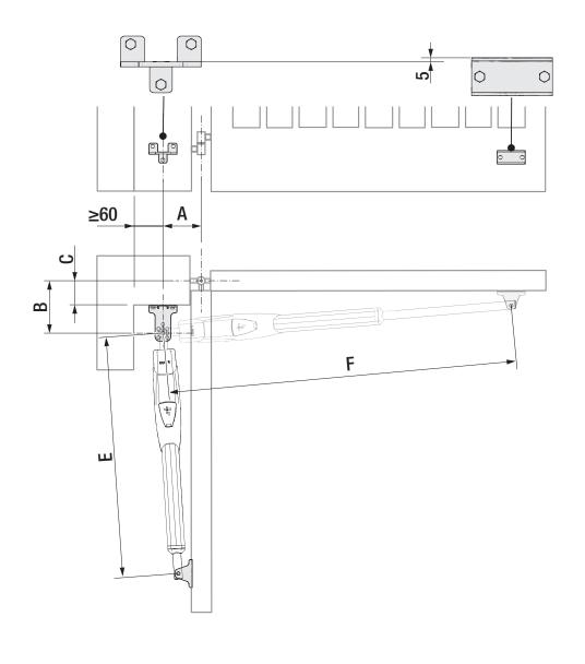
Identify the position where the gate bracket will be fixed (at a suitable height from the ground), then the position of the post bracket, respecting the measurements given in the figure below.
