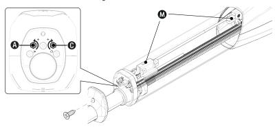
To move the microswitch 10 mm in either direction, turn the rod 12 times.
