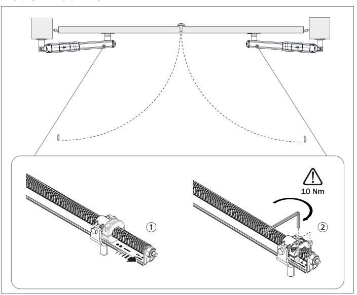
After adjusting the limit switch points, perform the travel teach-in following the instructions in the control panel manual.
