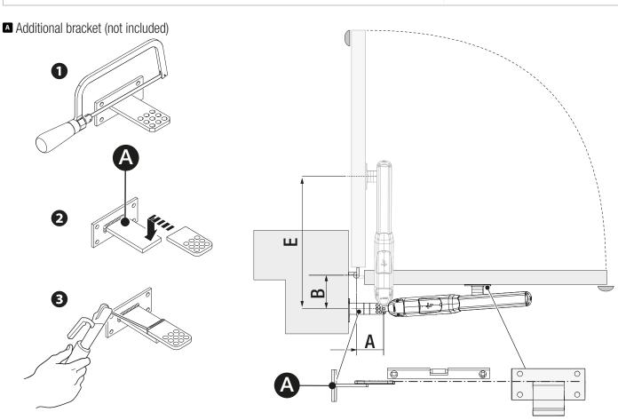
Respect the values indicated in the graphs. The graphs show the maximum opening angles in relation to the installation measurements A and B.
