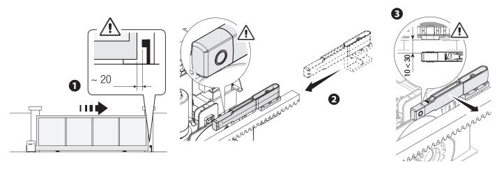
Fasten the support to the rack using the grub screws supplied.
