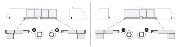
The figures below show the limit switch installed with the operator on the left.Installation of the limit switch on the right is symmetrical.
