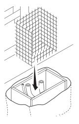
Insert the screws supplied in the anchoring plate. Lock the screws in place with the nuts supplied. Remove the pre-shaped clamps using a screwdriver. Fit the anchoring plate in the iron cage.
