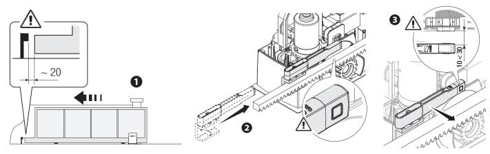
The limit-switch tab magnet must be perpendicular to the magnetic sensor.
