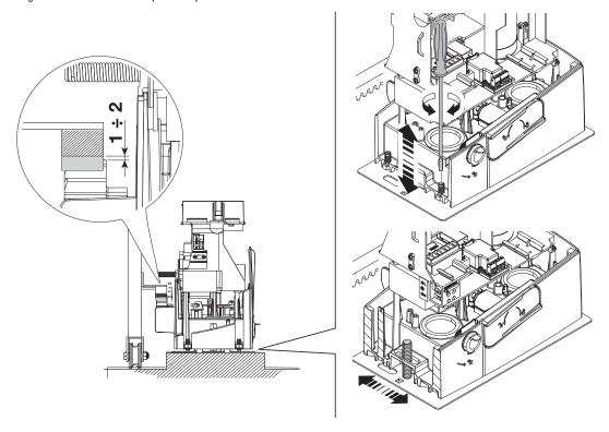
$\hfill \square$  Only fasten the operator after adjusting the pinion-rack coupling.
