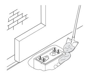
Remove the nuts from the screws.
