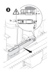
Fasten the support to the rack using the grub screws supplied.
