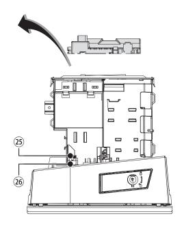
Remove the card cover before inserting the cards into the connectors.
