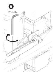
$\hfill\Box$  The tab magnet must be between 10 and 30 mm from the magnetic sensor.
