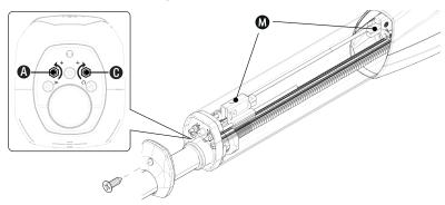
To move the microswitch 10 mm in either direction, turn the rod 12 times.
