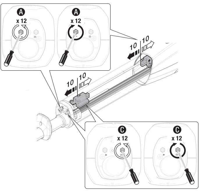
The travel end point adjustment procedure using a multimeter (tester) is described below. Alternatively, there is a specific tool available for adjusting the end point (code 801XC-0180).
