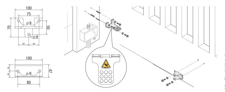
The self-locking nut must be loosely tightened so as not to affect the movement of the telescopic arm with the gate bracket.
