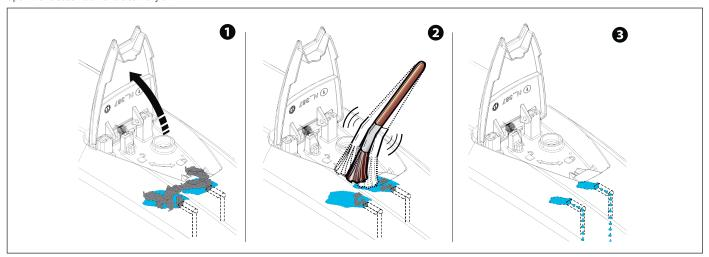
Grease the scraper ring on the end cap using EP2 grease.
