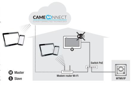
Single-family system with local power supplies and internal receiver connected in Wi-Fi
