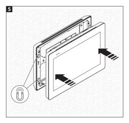
to make the device's installation more solid, use the supplied screws and dowels to fasten the frame to the wall.
