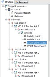
A call from the entry panel can ring a maximum of 20 devices (managed by the internal Master receiver of the apartment), whether they are connected to the LAN line or reachable from a Wi-Fi or mobile network using CAME Connect.
