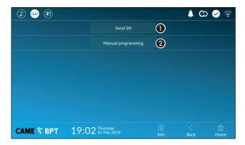
• This button is for sending the SN (serial number) to the Pcs/Xip software during the programming steps.
