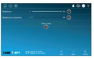
**1** Adjusts the brightness of the screen during use.
