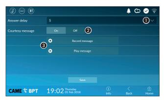
• From the drop down menu, select the ring time - expressed in seconds - after which the automatic recording is activated.
