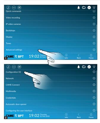
The section requires specific know-how in operating the video-intercom system. Wrong settings may cause partial or even total malfunctions; that is why the editing of some parameters is allowed only after entering the installer password; the default password is 112233).
