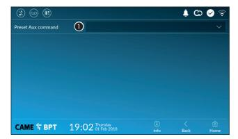
This window is for establishing which of the previously configured commands needs to be executed by pressing the Aux button on the homepage.
