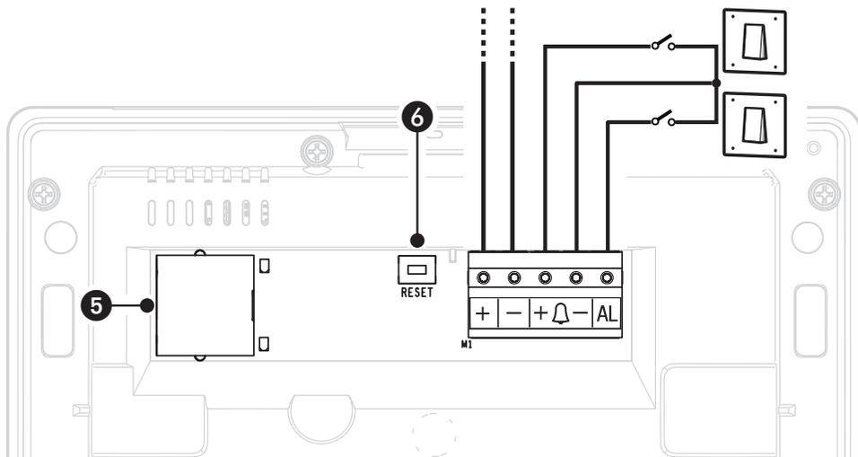
6 Reset button. When pressed it reboots the device; this operation DOES NOT require any deleting of programming.
