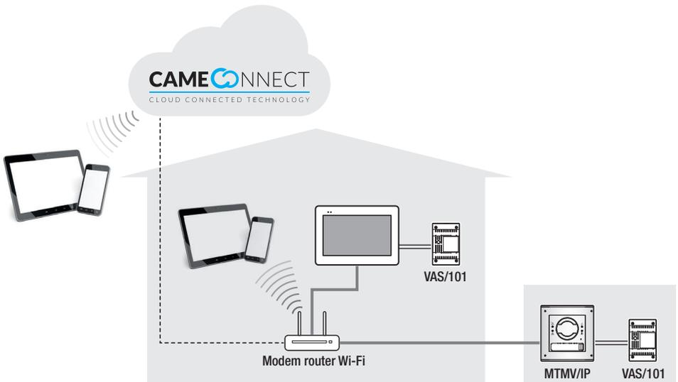
**Multi-family system with an internal receiver for each apartment; one of the receivers can be managed from a tablet or smartphone**
