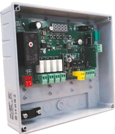
**RBE Plus** is the new control panel for access control, specifically for use with transmitters and all CAME CXN BUS accessories.
